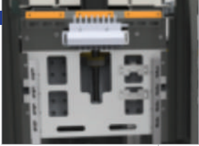
Z-axis adjustment for fabric thickness
